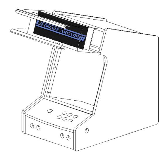
Using (2) 1" long wood screws (S1), attach 4 panel M's to panels A and B as show in the diagram below.
