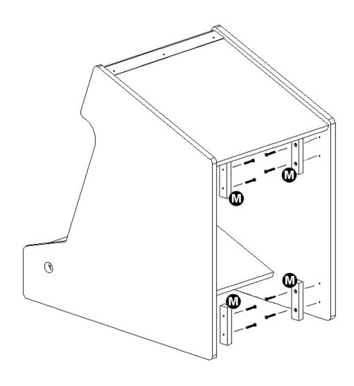
Using (3) 1" long wood screws (S1), attach both panel L's to panels A and B as show in the diagram below.
