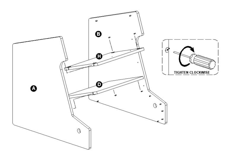
Attach panel F to panels A and B as show in the diagram below. Use a screwdriver and fully tighten each of the engaging cams.
